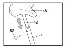
the Seat (48), dismount the exercise cycle, hold the Seat, and remove the Seat Knob (52). Raise or lower the Seat and insert the Seat Knob through the Frame (1) and the Seat Post (42). Tighten the Seat Knob into the welded nut on the Frame. **CAUTION: Make sure** to insert the Seat Pin through the Seat Post; do not insert the Seat Knob under the Seat Post.
